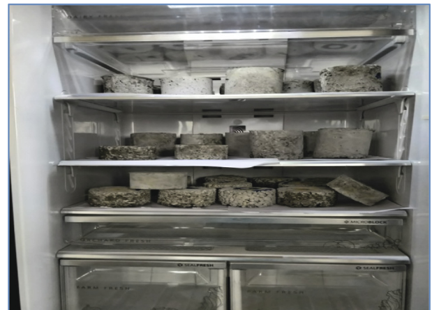
Fig. 2. Freezing and Thawing samples.
